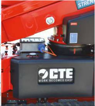
VALVE BLOCK PROTECTION KIT
